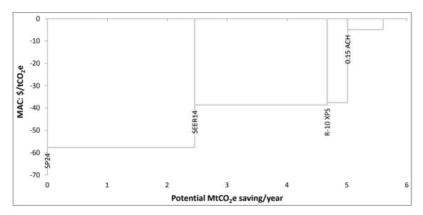
Figure 9. The MACC for electricity price 0.09 \$/kWh (SELECTED levers).
