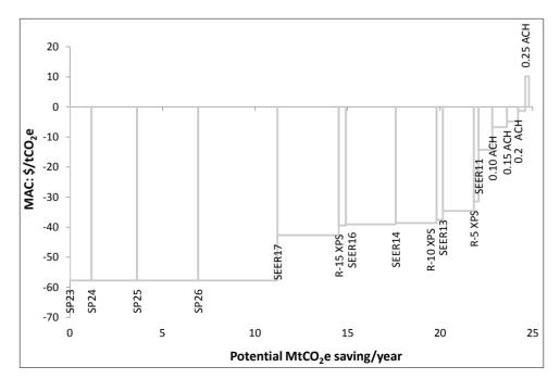
Figure 8. The MACC for electricity price 0.09 \$/kWh (ALL levers).
