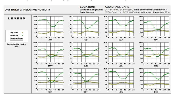
Figure 4. Monthly average profiles of temperature and humidity in Abu Dhabi.
