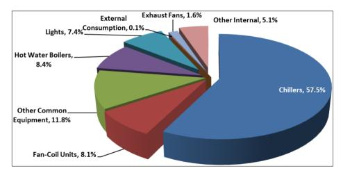
**Figure 3.** Contribution of air-conditioning load—driven by temperature, humidity and solar gains—to the electricity consumption profile for the year 2010 (1 January to 31 December). Note that a portion of the base-load is also due to air-conditioning (equipment running year-round).
