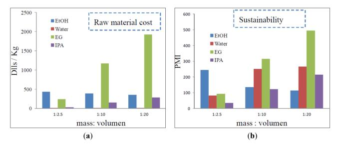
Figure 6. (a) Raw materials cost per kg of extract. (b) process mass intensity (PMI).
