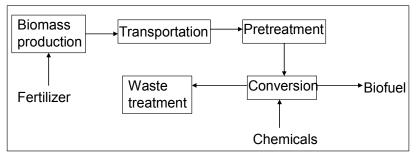
Ordinary bioconversion process for production of biofuel
