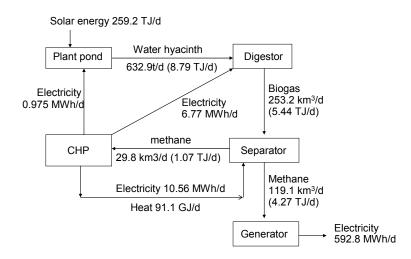
**Figure 2.** Average daily energy flow for the plantation of water hyacinth and digested to methane or further converted to electricity.
