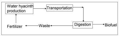
Integrated biomass production and digestion process for biofuel
