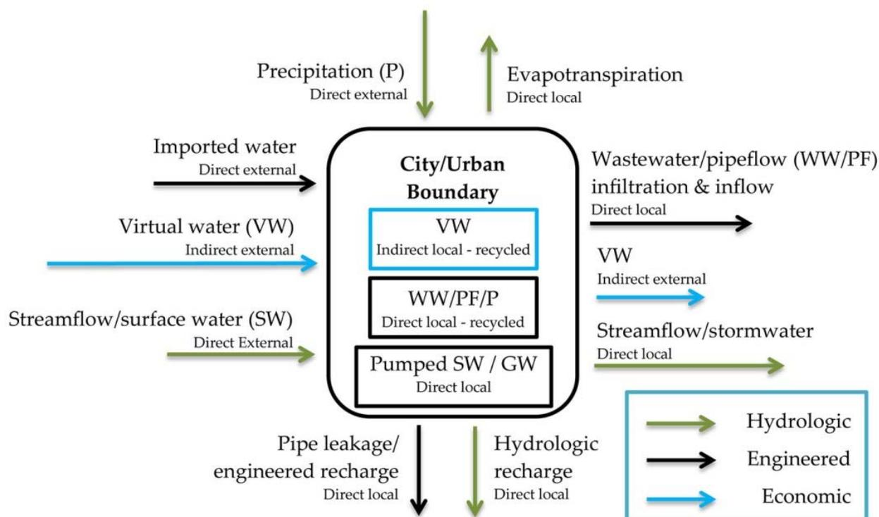
**Figure 1.** Conceptual diagram of the direct and indirect water flows of an urban area. The recycling of direct and indirect local water within the urban boundary is also identified. Flows are defined as local and external if they originate from within or outside the urban boundary, respectively. Flows are also identified as hydrologic, engineered, and economic.
