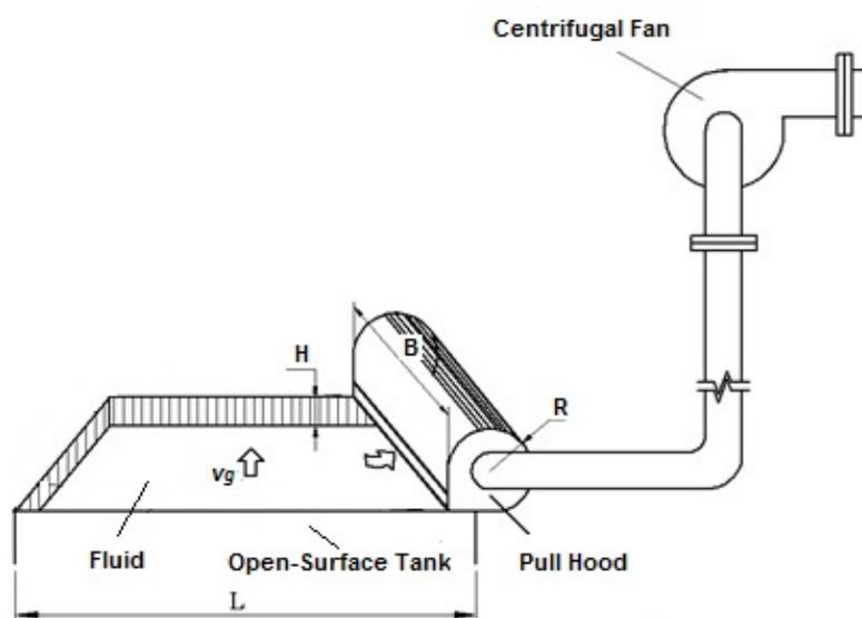
Figure 2. The push system and its geometric parameters.
