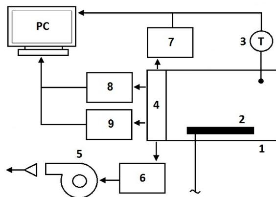
**Figure 1.** The schematic view of the test setup of the side absorber: 1 an open-surface tank; 2 a heater; 3 a thermometer; 4 a side absorber; 5 a fan; 6 a frequency drive; 7 a device for measuring pressure and flow velocity; 8 a gas density meter; and 9 a viscometer.
