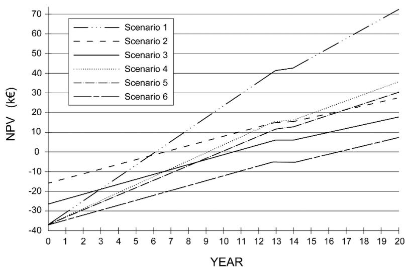
**Figure 4.** Evaluation of MH Floodlights replacement with LED Floodlights: trends of NPV in function of the time (investment by own funds,  $r = 2\%$ ).
