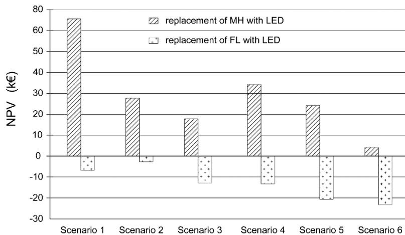
**Figure 5.** NPV values for MH floodlights and FL luminaires replacement with LED floodlight (investment by own funds,  $r = 2\%$ ).
