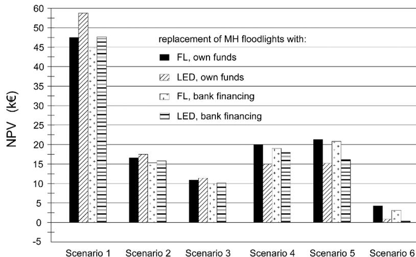
**Figure 6.** NPV values obtained for different MH floodlights replacement.
