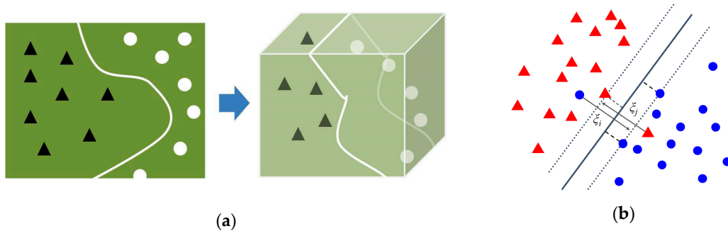
Figure 5. Explanation of the support vector machine (SVM) principle. (a) n -Dimensional hyperplane differentiating the two classes by the maximum gap; (b) non-separable case and the slack variables \xi_i [54].
