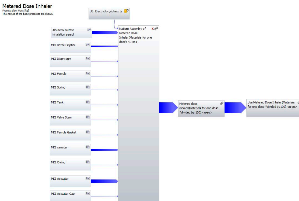
Figure S2. Life cycle assessment (LCA) inventory for the manufacturing and use of a metered dose inhaler (MDI).
