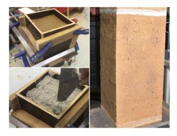
Figure 6. Prismatic specimen manufactured from Soil A, surfaced with a lime mortar.
