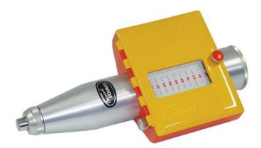
Figure 2. The original Schmidt series NR/LR (photo: Gilson company).
