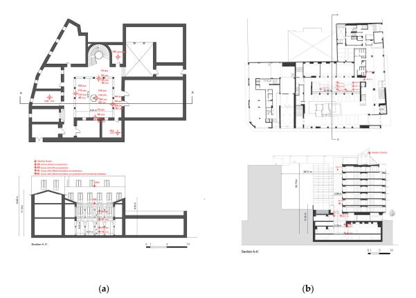
Figure 7. Floor plans and sections of the buildings in Cordoba (a) and Malaga (b) showing the data loggers' location.
