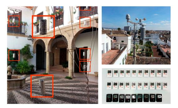
**Figure 8.** Monitoring campaign in Cordoba. (**Left**) data loggers in red boxes placed with sun protection elements to measure the air temperature; (**Right**) weather station on roof and data loggers.
