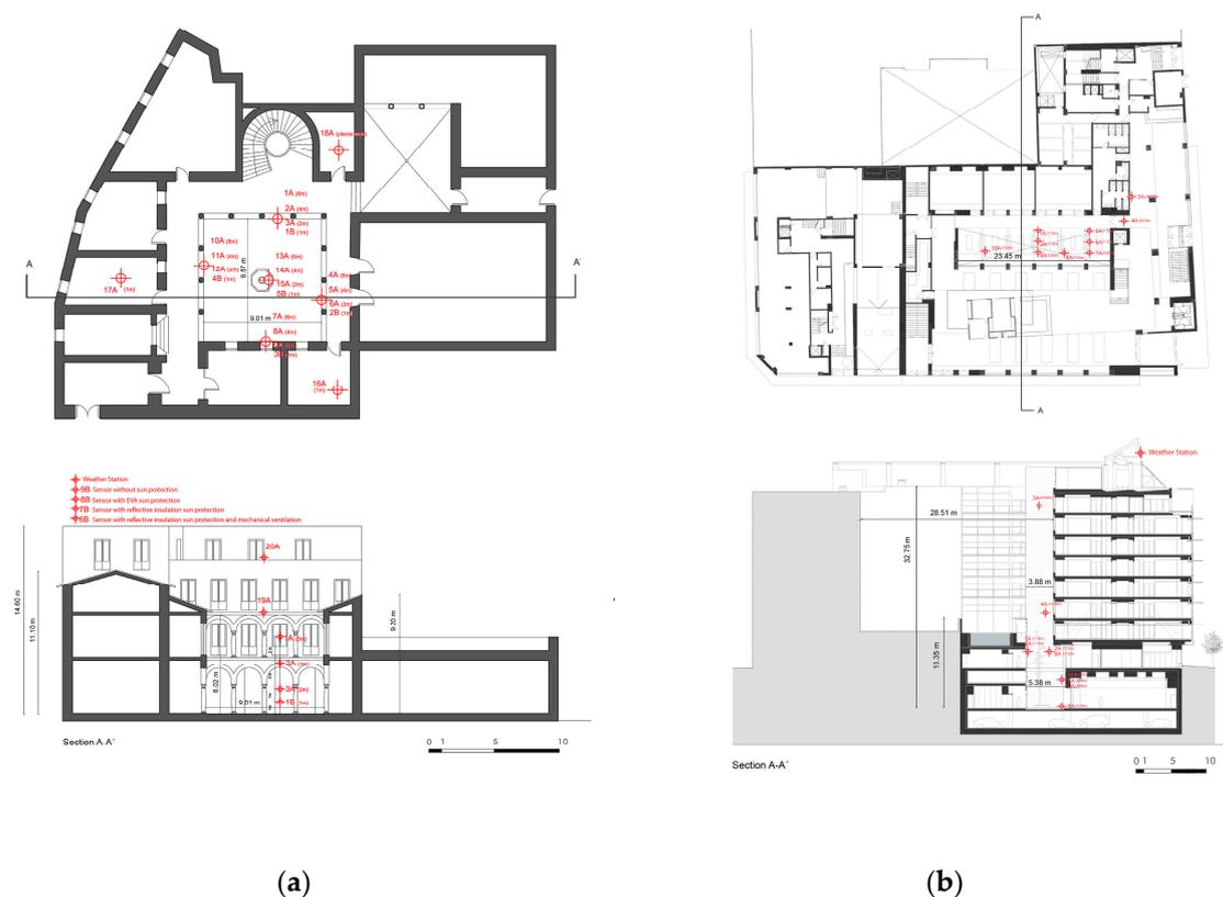
**Figure 7.** Floor plans and sections of the buildings in Cordoba (a) and Malaga (b) showing the data loggers' location.
