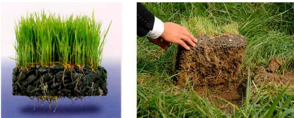
**Figure 1.** Photo of porous vegetation concrete blocks.
