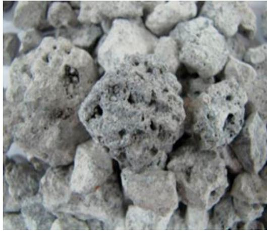
**Figure 2.** Photo of blast furnace slag aggregates.
