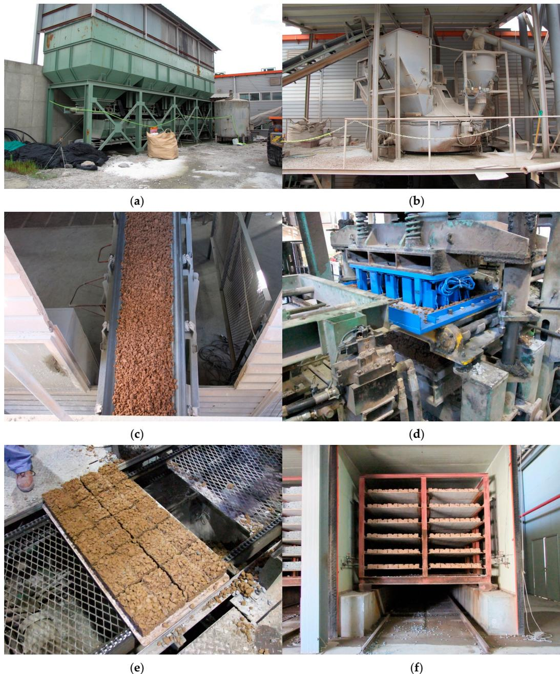
**Figure 8.** Manufacturing process of porous vegetation red clay green roof blocks. (a) Material supply; (b) mixing; (c) mixing materials transport; (d) forming; (e) product; (f) curing.
