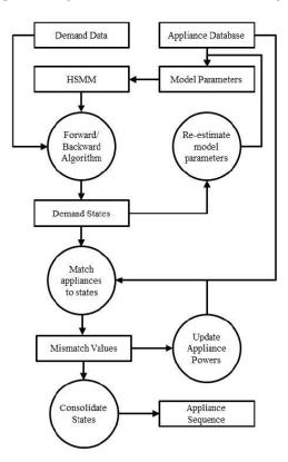
Figure 2. Process flow of demand disaggregation software tool.
