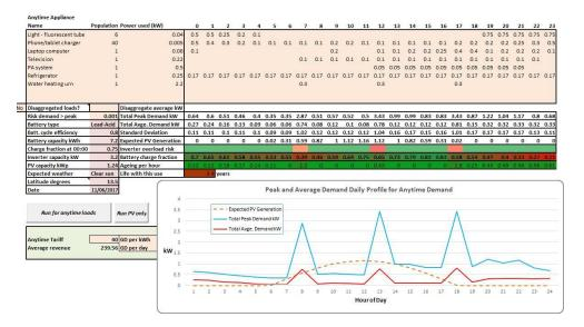
Figure 11. Initial load profile and battery condition model from The Gambia.
