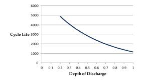
Figure 3. Wöhler curve for lead-acid battery based on depth of discharge.
