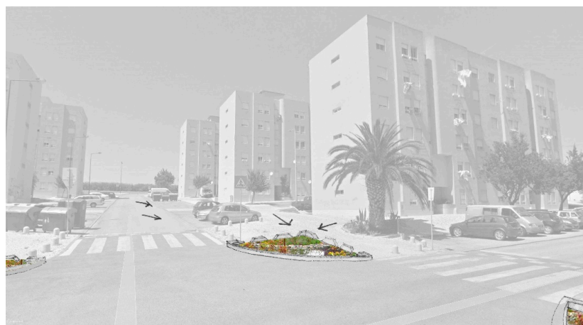
Figure A3. 3D sketch of the proposed rain gardens (and likely stormwater flow directions) to be implemented in a residential area at Carnide, namely at the intersection of Rua Professor Pais da Silva with Rua Professor Almeida Lima. Source: Author’s sketch.
