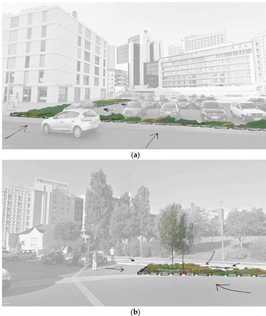
Figure A5. 3D sketches (a,b) of the proposed bioretention planters (and likely stormwater flow directions) to be implemented in a parking lot at Campolide, namely by the lower end of Rua de Campolide. Source: Author's sketch.
