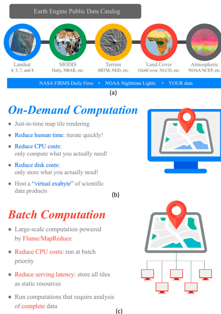
Figure 4. Google Earth Engine. (a) public data catalog, (b) on-demand, and (c) batch computation modes.
