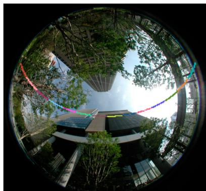
**Figure 3.** An example of a photo taken by the camera with a fisheye lens with the corresponding solar orbit diagram.
