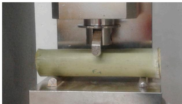
**Figure 4.** A three-point bending test on a bamboo specimen.
