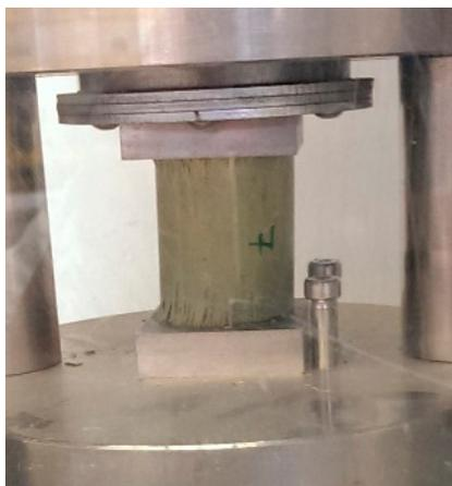
**Figure 3.** A bamboo specimen during the uniaxial compression test.
