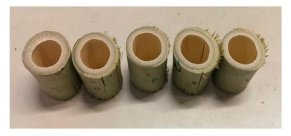
Figure 7. Specimens after compression tests.
