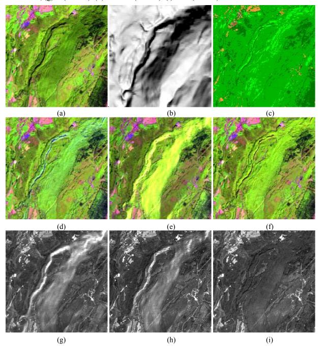
Figure 7 (a) presents the CV values for the classes 1 and 2. The average slope values are 19° (class 1) and 22° (class 2), not counting pixels in the flat plane. As low values indicate the best elimination of topographic features, the C method ranks first for the visible bands (1, 2), while C and MM achieve the same quality for the NIR and SWIR bands (3, 4). However, the visual comparison of Figure 1 (g),(i) clearly indicates a better performance of the MM algorithm.
