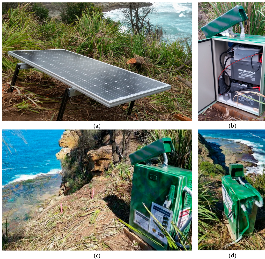
Figure 5. Camera setup on site showing (a) the solar panel; (b) the gel batteries, solar regulator, and power converters; and the cameras mounted in the security camera housings and the battery housing box for (c) the north camera and (d) the south camera.
