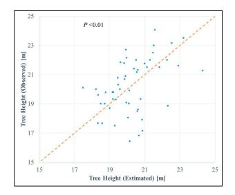
**Figure 4.** The relationship between estimated and observed tree heights. The dotted line in the center indicates 1:1. The Root Mean Square Error (RMSE) was calculated as 1.712 m ( $R^2 = 0.2076$ , linear trend).
