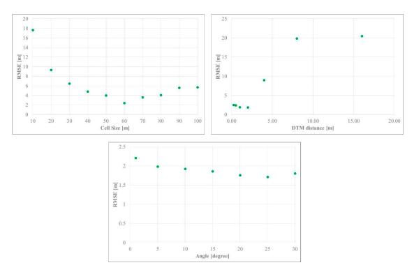
**Figure 2.** Root mean square error (RMSE) of tree heights in terrain models generated using various parameter settings to extract the ground points.
