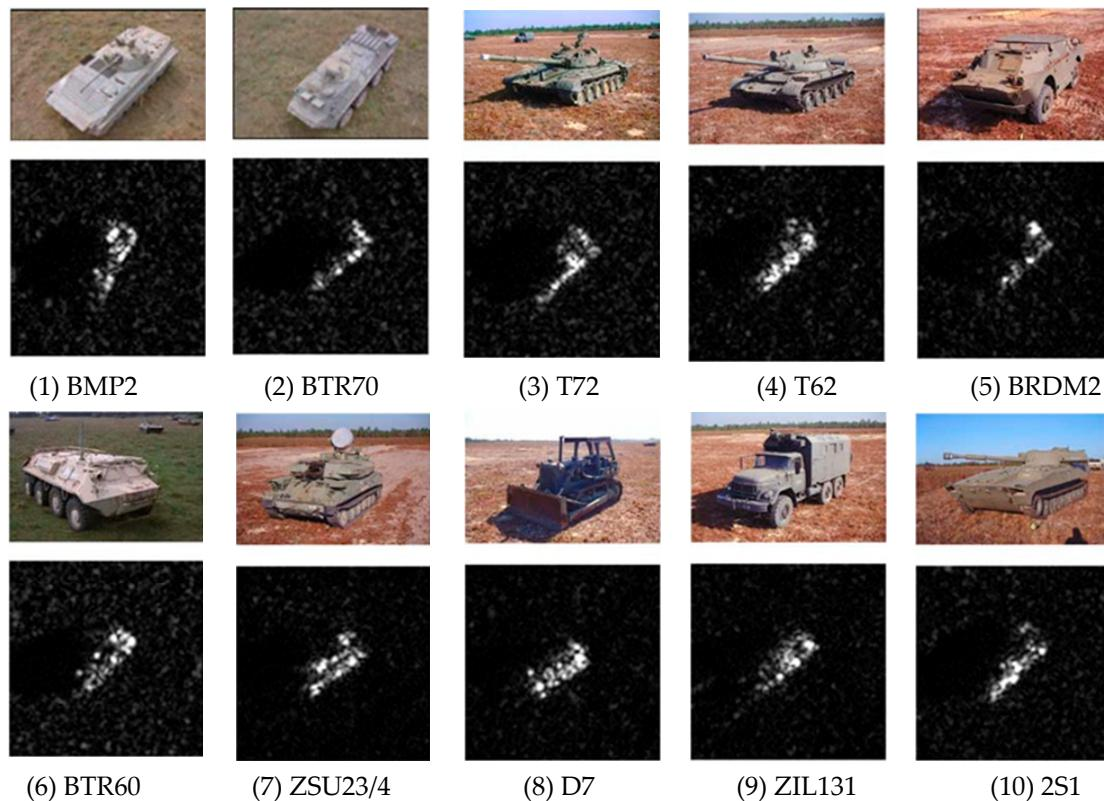
**Figure 6.** Types of military targets: (top) optical images; and (bottom) SAR images.
