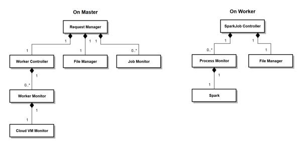
Figure 3. SparkCloud class diagram.
