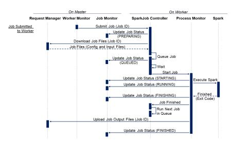
Figure 5. Worker-node sequence diagram.
