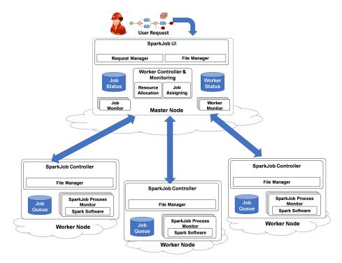
**Figure 1.** SparkCloud architectural components for master node and worker nodes. Master node manages user request allocations to different workers, which manage the execution of the simulation model on the basis of the request.
