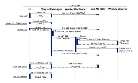
Figure 4. Master-node sequence diagram.
