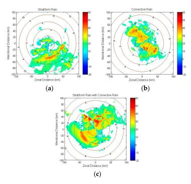
**Figure 3.** Dual-polarized radar PPI images of Z for (a) stratiform rain only, (b) convective rain only, and (c) stratiform rain together with convective rain.
