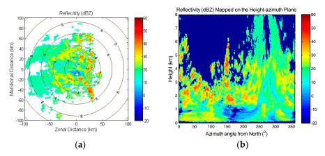
**Figure 10.** Radar reflectivity measured at 14:55 UTC on 14th June 2014 (a) PPI image (b) mapped on the height–azimuth plane.
