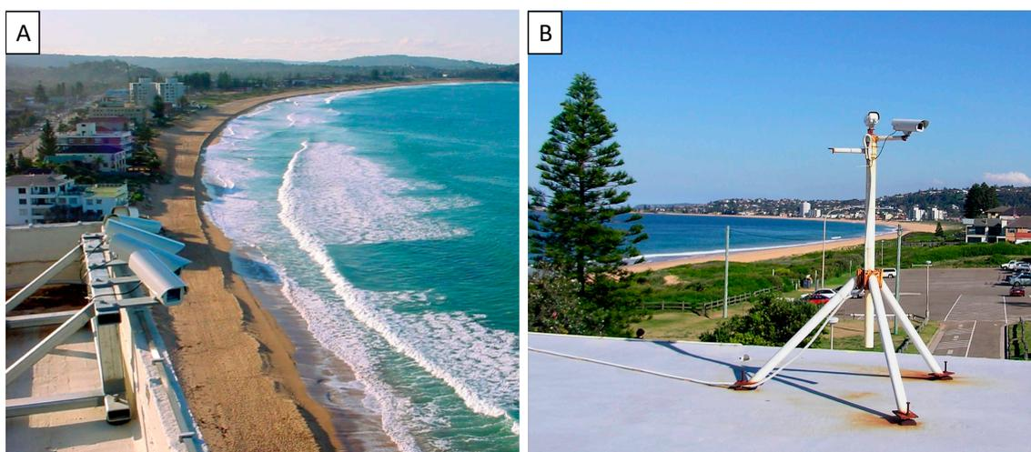
**Figure 6.** (A) The permanent Narrabeen Argus cameras system atop the Flight Deck Building that has been in operation since 2004. (B) The temporary North Narrabeen Argus cameras installation atop the North Narrabeen Surf Life Saving Club, that operated between 2005–2008.
