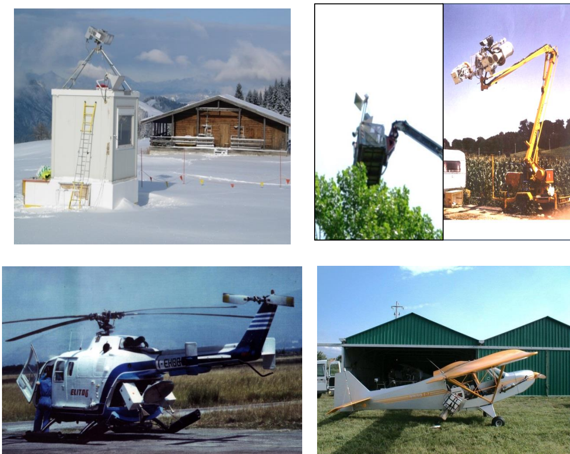
Figure 1. Installations of IROE microwave radiometers on several platforms: in a shelter on snow, on hydraulic booms on forest and agricultural fields, and on helicopter and ultra-light aircraft.
