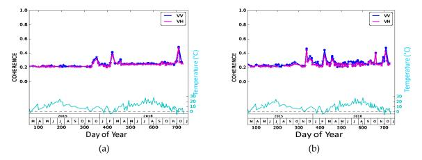
**Figure 7.** Temporal profiles of  $|\rho|$  observed over an oak (**a**) and a pine (**b**) stand with VV and VH polarization. *In situ* temperatures at 2 m are also shown (cyan).
