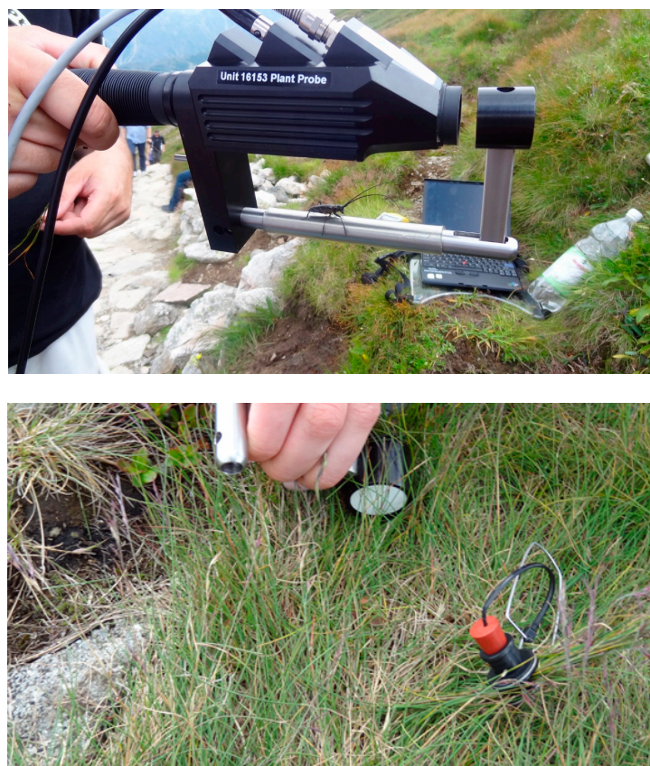
Figure 3. Hyperspectral measurements by ASD PlantProbe (upper picture), which is connected to the ASD FieldSpec by an optical fiber cable (black one on the upper picture). A closed leaf clip (picture lower part) is used for adapting leaves to the darkness before measurements of chlorophyll fluorescence.
