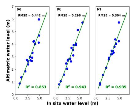
**Figure 4.** Results of the comparison between the altimetry-based water stages from ENVISAT on its second orbit for (**a**) Station 1, (**b**) Station 2 and (**c**) Station 3 and the in-situ ones from Lambaréné gauge station.
