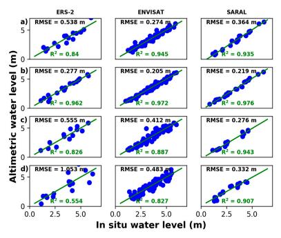
**Figure 3.** Results of the comparison between the altimetry-based water stages from ERS-2/ENVISAT/ SARAL for tracks 401 (**a**), 902 (**b**), 945 (**c**), 444 (**d**) and the in situ ones from Lambaréné gauge station.
