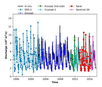
**Figure 11.** Time series of river discharge at Lambaréné from the in-situ gauge record (black continuous line), the multi-mission altimetry-based record (ERS-2 data are represented with diamonds, ENVISAT with blue crosses on its nominal orbit and with green triangles on its second orbit, Cryosat-2 with green-blue stars, SARAL with red circles, Sentinel-3 with purple dots).
