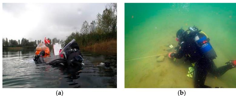
**Figure 11.** Photographs of the underwater survey operation in Lago Tramonto, Gambulaga, Portomaggiore (FE, Italy): (a) Setting of the equipment before the survey; (b) Pegging the underwater topographical reference point (photo by Antonio Duccoli and Paolo Farina).
