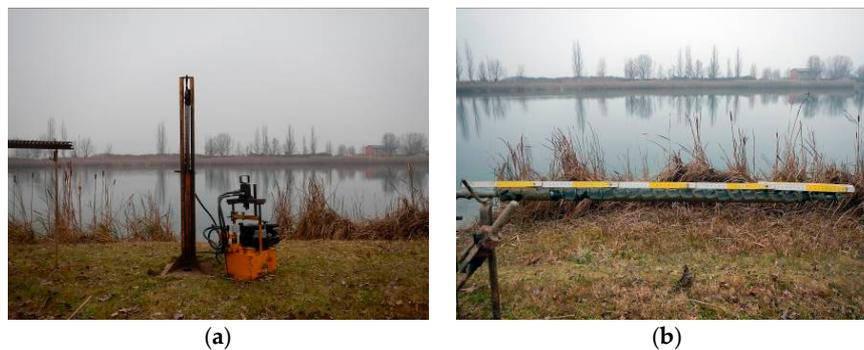
**Figure 10.** Drilling No. 1 in 2017 in Lago Tramonto, Gambulaga, Portomaggiore (FE, Italy): (a) The drilling machine; (b) Work in progress while drilling, sediment check (photo by Giovanna Bucci).
