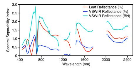
**Figure 7.** Spectral separability indices between green and brown for leaf (red line) and canopy (blue line) reflectance spectra. The separability index for canopy reflectance following brightness normalization (BN) is also provided (cyan line).
