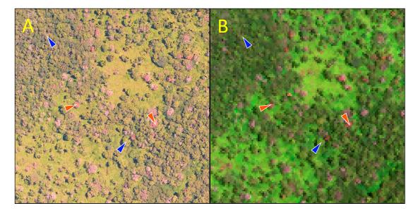
**Figure 2.** Example images from the Carnegie Airborne Observatory: (**A**) high-resolution digital color camera and (**B**) visible-to-shortwave infrared (VSWIR) imaging spectrometer showing suspected ROD-infected brown-state crowns and green crowns. Red arrows point to representative brown-state trees and blue arrows point to healthy green trees.
