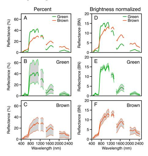
**Figure 6.** Comparisons of mean green and brown canopy reflectance and brightness-normalized canopy reflectance are shown in (**A**,**D**), respectively, followed by mean, minimum and maximum reflectance values for green (**B**,**E**) and brown (**C**,**F**) foliage.
