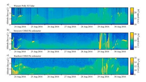
**Figure 2.** Remote 24/7 measurement conducted on 24–30 August 2016. Range and background corrected signal at 1064 nm of (**a**) the PollyXT lidar at the RT-Lab in Warsaw (central Poland) and (**b**) CHM15K ceilometer measurements at SolarAOT Observatory in Strzyzow (south-eastern Poland) and (**c**) IGF-PAS Observatory in Raciborz. High signal intensities are denoted with the yellow colour and low with blue. Note different scale of the plots.
