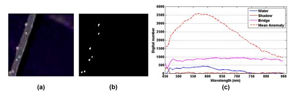
**Figure 3.** (**a**) The image scene of PaviaC dataset by the ROSIS sensor; (**b**) ground truth map of 47 pixels representing anomalies; and (**c**) spectral curves of background and average anomalous signature.
