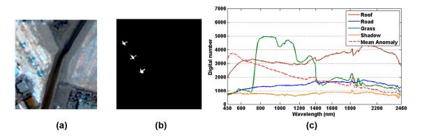
**Figure 4.** (**a**) The image scene of San Diego dataset by the AVIRIS sensor; (**b**) ground truth map of 58 pixels representing anomalies; and (**c**) spectral curves of background and average anomalous signature.
