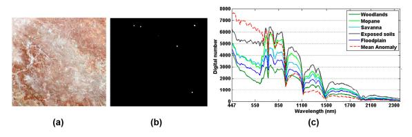
**Figure 5.** (**a**) The image scene of Botswana dataset by the EO-1 Hyperion sensor; (**b**) ground truth map of 35 pixels representing anomalies; and (**c**) spectral curves of background and average anomalous signature.
