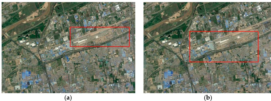
**Figure 10.** False detection result in an image with no airport in it. (a) Faster R-CNN; (b) LSD + AlexNet. [Image courtesy of Google Earth].
