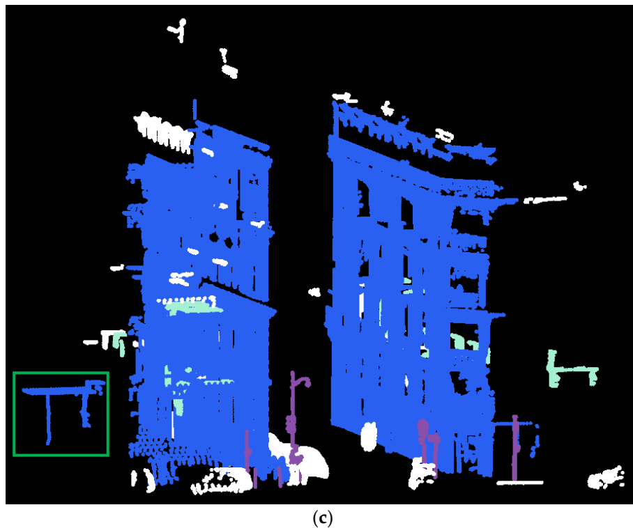
Figure 20. The pole-like road furniture detection from the Paris dataset. (a) the ground points and above-ground components; (b) the detected façade (light blue) and road furniture (purple). The entities behind façades were incorrectly detected as road furniture in the left green frame; (c) the label of incorrectly detected pole-like objects inside the buildings in the left green frame were redressed after occlusion analysis.
