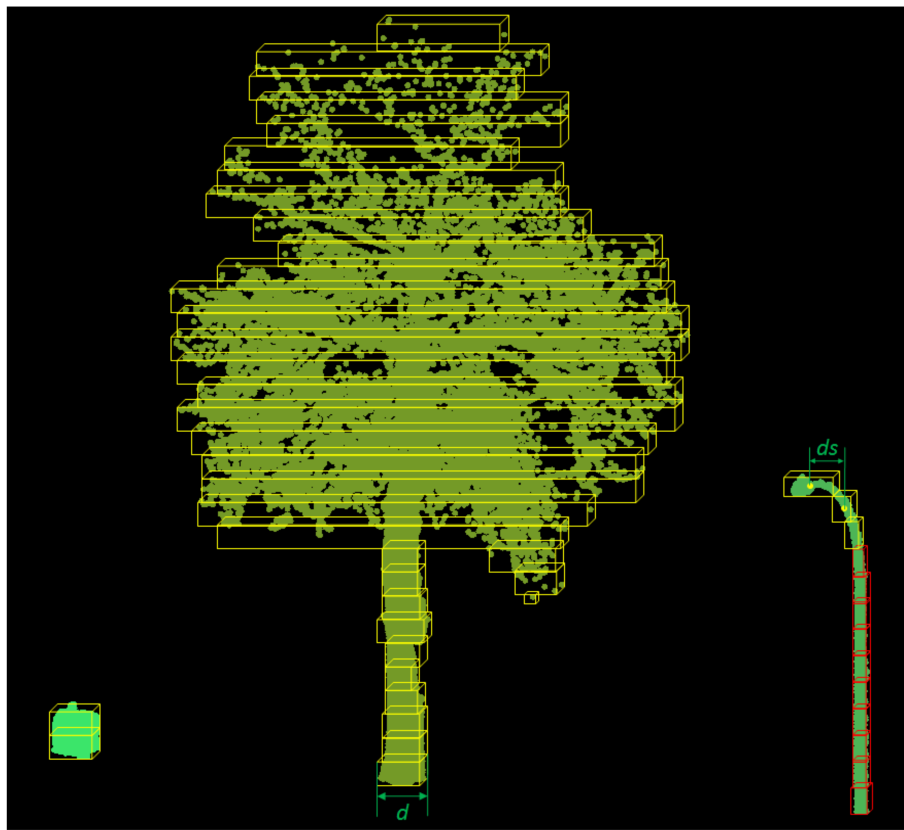
Figure 4. The slice-based detection of pole-like road furniture.
