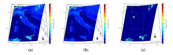
**Figure 4.** Steps to obtain High Resolution Visible channel (HRV)Long Term Temporal Test (LTTT) product: (a) HRV Reflectance over land, 2017-04-10 07:45 UTC; (b) Clear sky reference map; (c) HRV Reflectance over land, cloudy areas.
