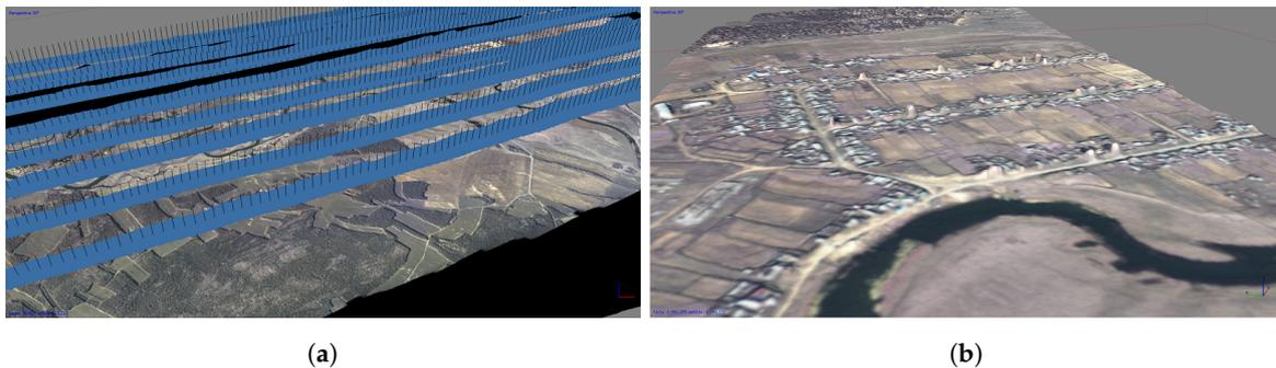
**Figure 3.** Processing of the frame images using Agisoft Photoscan: (a) alignment of frames and computation of the orthophoto; and (b) computation of the DEM of the area (Selenga Delta Village).
