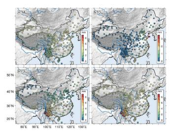
**Figure 2.** RMS of the vertical displacements due to ATML, NTOL, HYDL, and their sum (SumL), predicted with GFZ loading products for the CMONOC stations.
