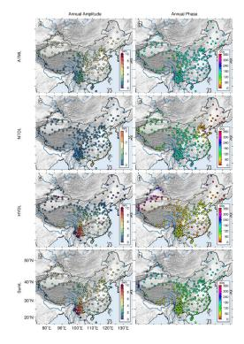
**Figure 4.** Vertical annual amplitudes and phases of the ATML (**a**,**b**), NTOL (**c**,**d**), HYDL (**e**,**f**), and SumL (**g**,**h**) time series predicted with GFZ loading products for the CMONOC stations. The annual phase is the day of year when an annual signal reaches its maximum.
