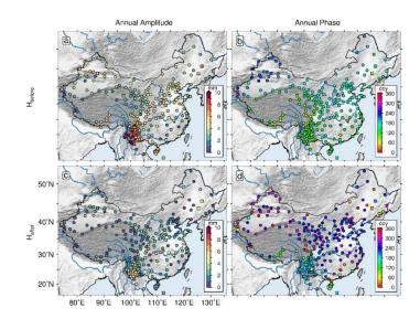
**Figure 5.** Vertical annual amplitudes and phases of the  $H_{before}$  (**a**,**b**) and  $H_{after}$  (**c**,**d**) time series for the CMONOC stations. The annual phase is the day of year when an annual signal reaches its maximum.
