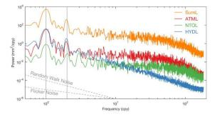
**Figure 11.** Stacked power spectra of the vertical displacements due to ATML, NTOL, HYDL, and SumL for the selected 208 CMONOC-II stations. The stacked power spectrum of SumL has been shifted upward for clarity (by a factor of 100). Vertical gray lines indicate the annual and semiannual oscillations.
