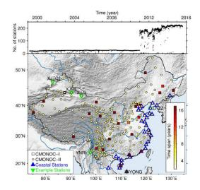
**Figure 1.** Geographical distribution and time spans of the selected 235 CMONOC stations used in this paper. The CMONOC-I (**square**) and CMONOC-II (**circle**), two subnetworks of the CMONOC, are composed of 27 and 208 stations, respectively. The blue triangles indicate 34 coastal stations located within 100 km distance of coast. The green inverted triangles indicate six selected representative stations.
