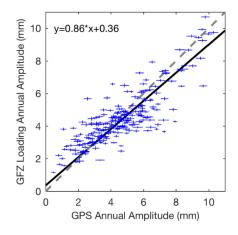
**Figure 6.** Comparison of vertical annual amplitudes between the  $H_{before}$  and SumL time series. The gray dashed line indicates perfect match. The black line indicates the best fit line estimated with a weighted total least squares algorithm.
