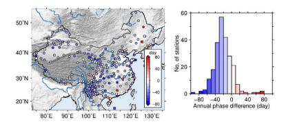
**Figure 7.** Phase differences between the vertical annual signals of SumL and H<sub>before</sub> time series (**left panel**) and its histogram (**right panel**).
