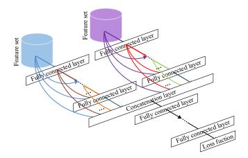
Figure 5. The overall architecture of the two-stream deep feature fusion model.
