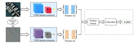
**Figure 2.** The texture coded two-stream deep architecture. The raw RGB network stream takes RGB images as input. The mapped LBP coded network stream takes mapped LBP images as input. Two different sets of features are fused using the two-stream deep feature fusion model.
