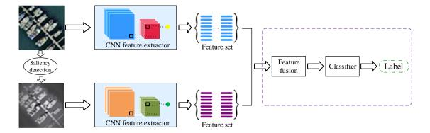
**Figure 4.** The saliency coded two-stream deep architecture. The raw RGB network stream takes RGB images as input. The saliency coded network stream takes the processed images through saliency detection as input. Two different sets of features are fused using the two-stream deep feature fusion model.
