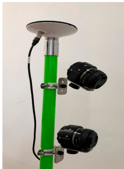
Figure 4. Two CCD lens placement details.
