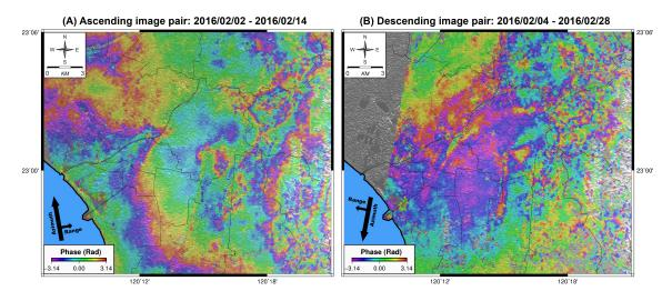
**Figure 2.** Coseismic interferometric results in Tainan City. (**A**) The results of ascending image pairs. The master image 2016/02/02, and the slave image was 2016/02/14. (**B**) The results of descending image pairs. The master image was 2016/02/04, and the slave image was 2016/02/28. There are some small and clear fringes (diameters are from 1 km–3 km) that exist in study area. The time format of acquisition for the SAR image is provided as YYYY/MM/DD.
