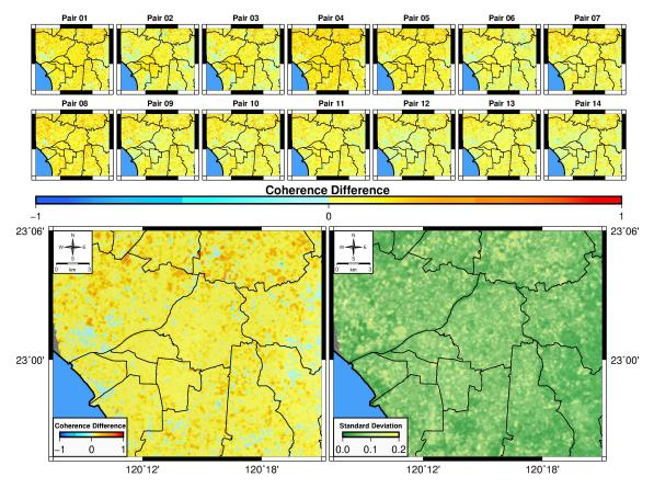
**Figure 6.** The background coherence difference results for ascending orbits. The top two rows are the time series of coherence differences for the ascending background image pairs. The subfigure in the lower-left quarter displays the mean values of coherence differences for ascending background image pairs. The subfigure in the lower-right quarter shows the values of standard deviations for ascending background image pairs.
