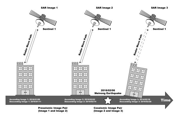
**Figure 3.** Conceptual diagram that shows the decrease of coherence before and after an earthquake. SAR: synthetic aperture radar.
