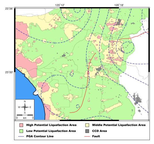
**Figure 9.** The comparison of CCD with liquefaction potential and peak ground acceleration (PGA) maps. The dark gray areas show the CCD results. The liquefaction potential map was classified into three categories. The high, middle and low potential areas are marked as red, yellow and green, respectively. The blue dashed lines are the PGA contour map (modified from Wu et al. [4]).
