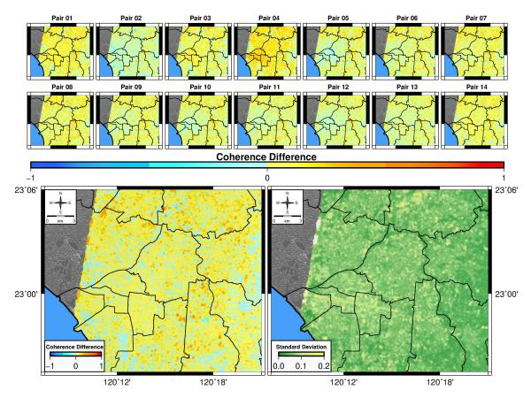
**Figure 7.** The background coherence difference results for descending orbits. The top two rows are the time series of coherence differences for the descending background image pairs. The subfigure in the lower-left quarter displays the mean values of coherence differences for descending background image pairs. The subfigure in the lower-right quarter shows the values of standard deviations for descending background image pairs.
