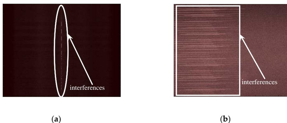
**Figure 1.** Synthetic Aperture Radar (SAR) echoes corrupted with (a) and (b) narrow-band interference (NBI) in range-frequency azimuth-time domain and wide-band interference (WBI) in azimuth-frequency range-time domain.
