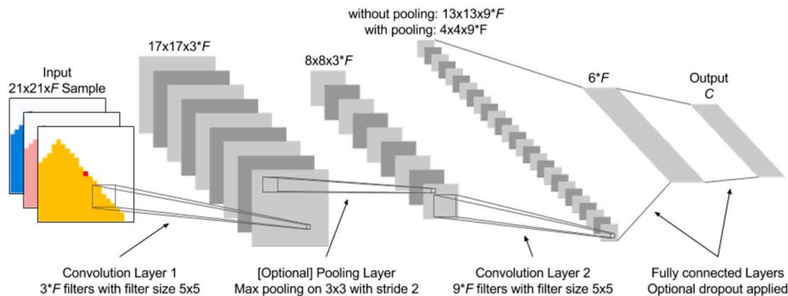
**Figure 3.** Structure of convolutional neural network (CNN) for classification of tree species. The variable  $F$  denotes the dimension of the input feature space.
