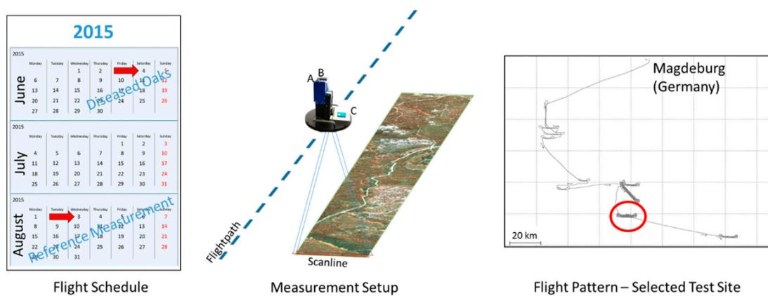
**Figure 1.** Left: Calendar depicts the dates and scopes of the measurement flights. Middle: Measurement setup for hyperspectral imaging data: (A) Hyspex VNIR 1600, (B) Hyspex SWIR 320m-e, and (C) Novatel SPAN CPT inertial measurement unit (IMU) mounted on stabilized platform (not depicted). Images have been recorded at an altitude of ~1000 m above ground level with FOV of 17° (VNIR) and 14° (SWIR). Right: Trajectory of the flight on 3 August.
