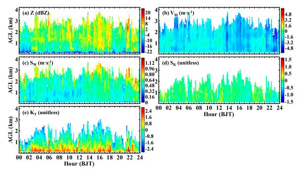
resulting in obtuse radar spectra. In contrast, the lower part of the cloud has a positive  $K_T$  due to raindrop rapid collision and coalescence processes, resulting in peaky radar spectra [38,64].
