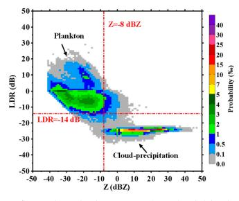
**Figure 3.** Ka-MMCR reflectivity-linear depolarization ratio (Z-LDR) probability distributions for warm clouds and precipitation and plankton. A couple of Z and LDR thresholds were set to -8 dBZ and -14 dB to eliminate the plankton.
