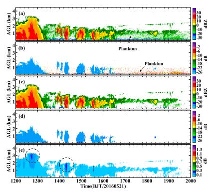
**Figure 5.** Time–height cross sections of the original reflectivity (**a**), original linear depolarization ratio (**b**), reflectivity after QC (**c**), linear depolarization ratio after QC (**d**), and the deviation (**e**) between (**a**) and (**c**), as observed by Ka-MMCR on 21 May 2016.
