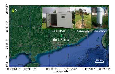
**Figure 1.** Experimental location of the Longmen Weather Observatory (LM, 23.783°N, 114.25°E, 86 m above sea level) and Ka-MMCR, disdrometer, and ceilometer (CL) instruments.
