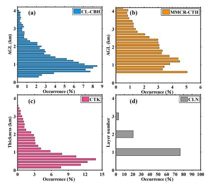
**Figure 13.** Occurrences of ceilometer (CL)-measured cloud base height CBH (**a**), Ka-MMCR-derived cloud top height CTH (**b**), synthetic cloud thickness CTK (**c**), and cloud layer number CLN (**d**), at different height levels.
