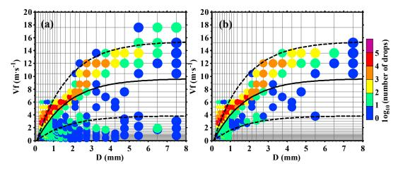
**Figure 6.** Raindrop diameter (D) -falling velocity ( $V_f$ ) frequency distributions before (**a**) and after QC (**b**) for the entire PARSIVEL dataset. D represents the raindrop diameter,  $V_f$  is the raindrop falling velocity, and the solid line represents the D-V<sub>f</sub> theoretical relationship under a still air condition.
