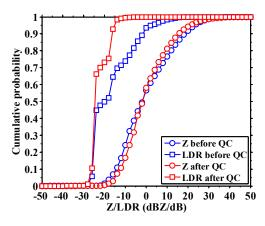
**Figure 4.** Cumulative probability curves of Ka-MMCR reflectivity (Z) and linear depolarization ratio (LDR) before and after data quality control (QC).
