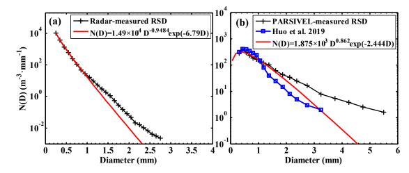
**Figure 15.** Average raindrop size distributions derived from the radar Doppler spectra (**a**) overhead and observed by PARSIVEL on the ground (**b**). The red lines are the fitted gamma distribution.
