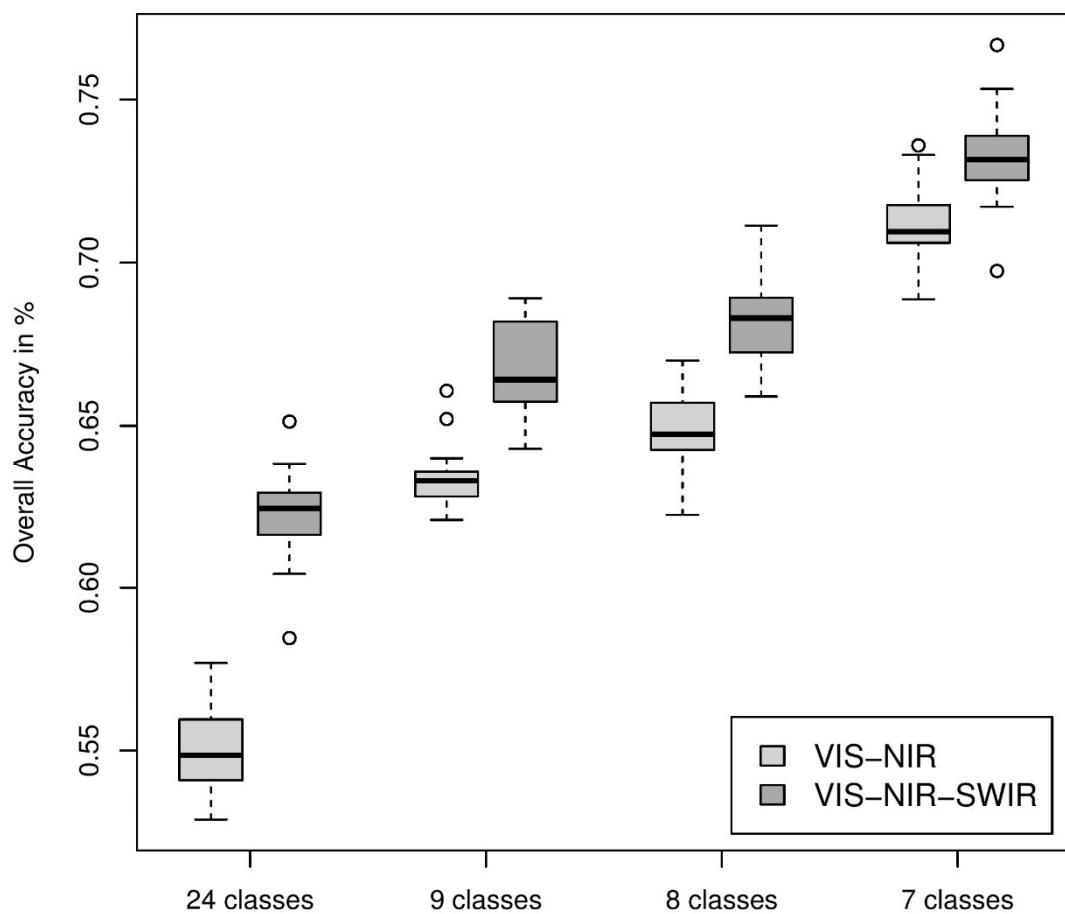
**Figure 1.** Achieved overall accuracies for the classification of different aggregation levels for land cover classes, VIS-NIR (SPOT6) compared to the multi-band VIS-NIR-SWIR product.
