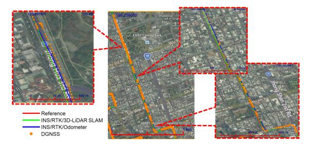
**Figure 11.** Scenario 1: zoomed GNSS-hostile area with severe multipath interference or non-line-of-sight (NLOS) reception.
