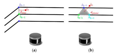
**Figure 4.** Geometric relationship for extracted features: (a) edge line for an edge point, (b) planar surface for a planar point.
