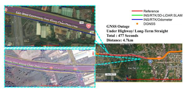
**Figure 15.** Scenario 2: zoomed area underneath the highway with long-term straight movement without a GNSS solution.
