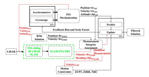
**Figure 1.** Flowchart of the inertial navigation system (INS)/ global navigation satellite system (GNSS)/3D light detection and ranging-simultaneous localization and mapping (LiDAR-SLAM) fusion design.
