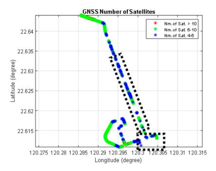
Figure 8. Differential GNSS solution encoded by the number of satellites in an urban area.
