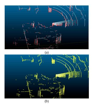
Figure 3. Demonstration of feature extraction: (a) edge points (red), (b) planar points (yellow).
