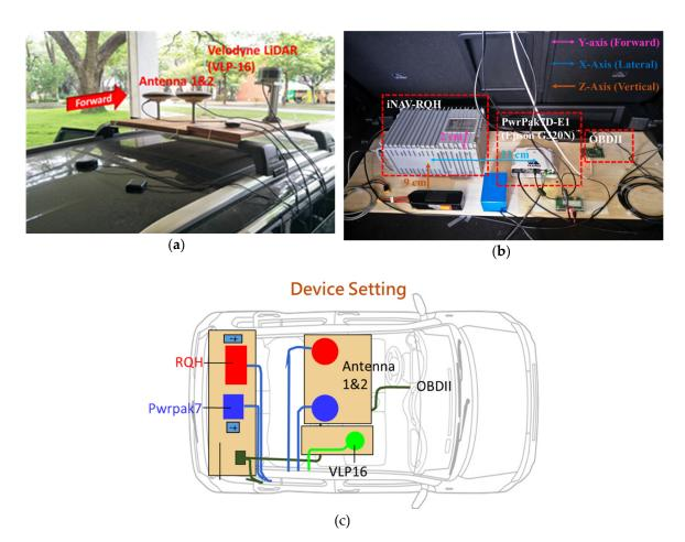
**Figure 7.** Configuration of the designed land vehicle: (a) GNSS antennas and LiDAR, (b) inertial measurement units (IMUs), (c) device setting.
