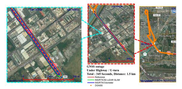
Figure 14. Scenario 2: zoomed area underneath the highway with a long-term GNSS outage and U-turn.
