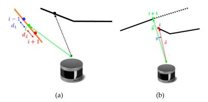
**Figure 2.** Unreliable extraction from two situations: (a) roughly parallel situation, (b) occluded situation.
