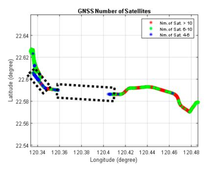
**Figure 9.** Differential GNSS solution encoded by the number of satellites in a highway area.
