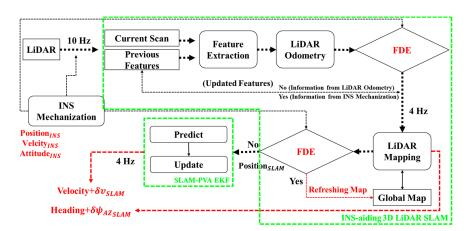
**Figure 6.** Structure of the proposed INS-aiding 3D LiDAR-SLAM and SLAM-position velocity acceleration (PVA) extended Kalman filter (EKF).
