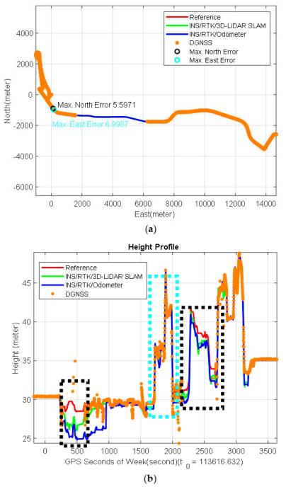
Figure 13. Scenario 2 results: (a) horizontal trajectory, (b) height profile.
