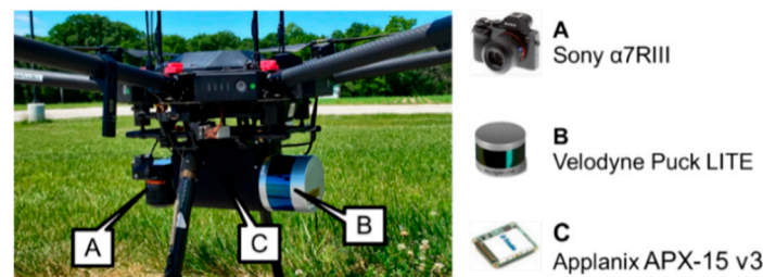
Figure 2. The unmanned aerial vehicle (UAV)-based mobile mapping system and onboard sensors used in this study.
