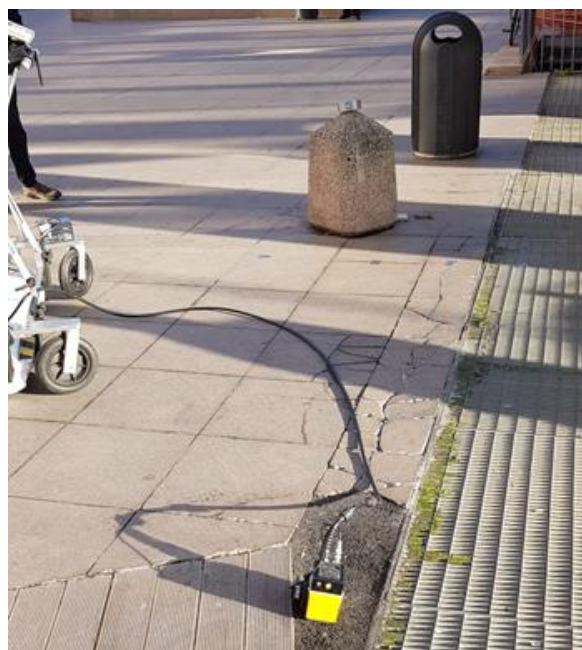
Figure 3. A photograph of the exploited GPR antenna.
