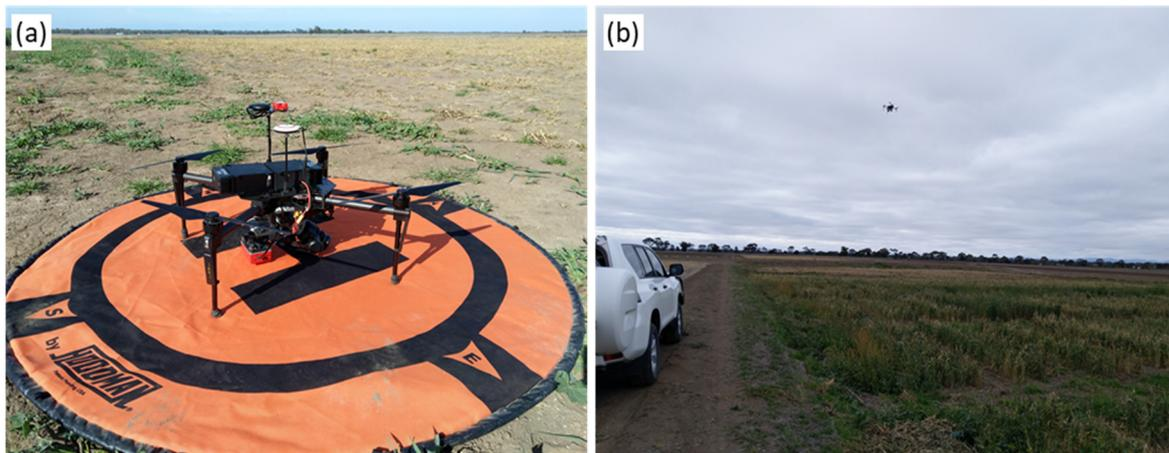
**Figure 1.** Field high-throughput phenotyping: (a) Unmanned aerial vehicle mounted with a RedEdge MicaSense multispectral camera, a global positioning system and downwelling light sensor; (b) Aerial mission on a field experiment at Plant Breeding Centre, Horsham, Victoria, Australia.
