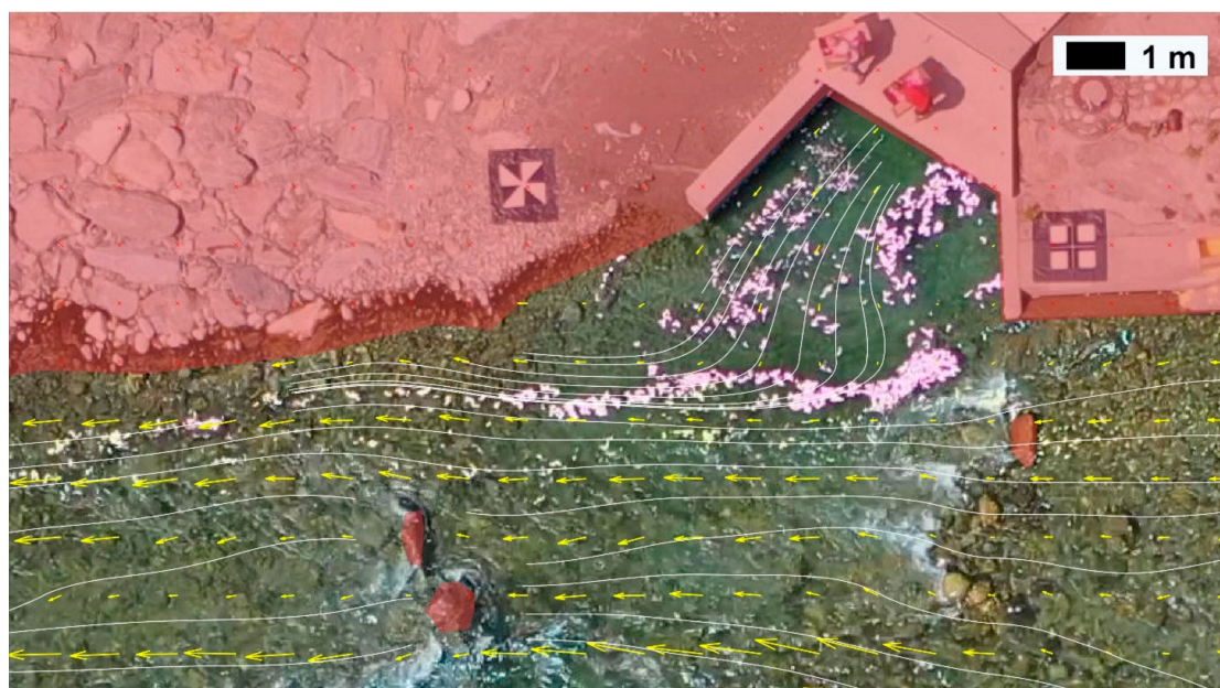
Figure 6. A flow pattern near the fishway calculated with the use of large IA: 96/96 px in the first pass and 96/48 px in the second pass.
